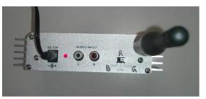
All transmitters must be plugged in at the same time to ensure synchronization. This will eliminate any interference. When plugged in, the red light next to the power in plug must light up as shown.
